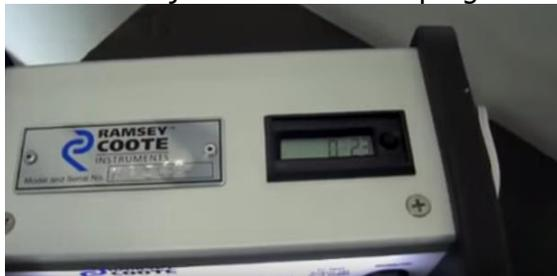
To turn the alarm off, turn the red switch on the control unit (the alarm) to the "Off" position. The bell sound ceases ringing and the timer stops so the time can be recorded.
